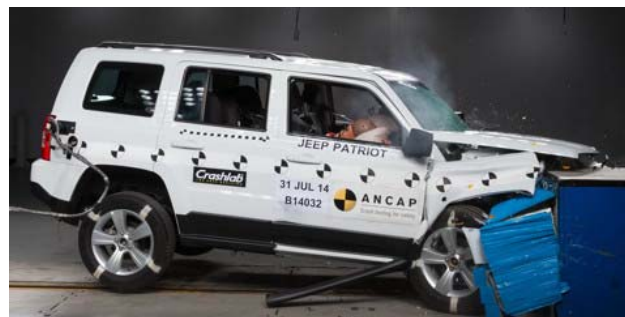
Frontal offset test at 64 km/h
