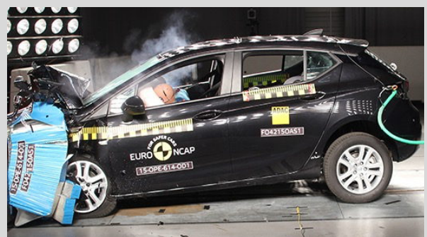
Frontal offset test at 64km/h
