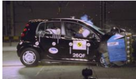
Offset crash test at 64km/hr
