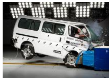
Offset crash test at 64km/hr
