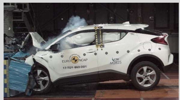
Frontal offset test at 64km/h
