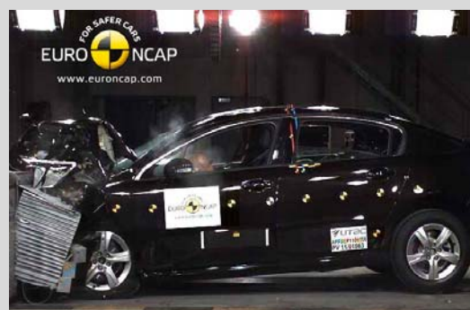
Frontal offset test at 64km/h
