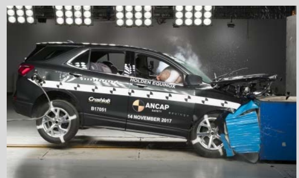
Frontal offset test at 64km/h
