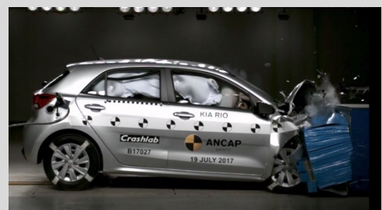
Frontal offset test at 64km/h
