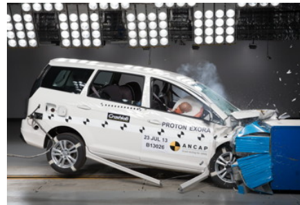
Frontal offset test at 64 km/h
