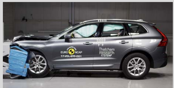
Frontal offset test at 64km/h
