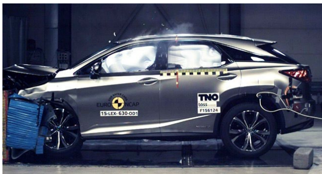
Frontal offset test at 64km/h (Euro NCAP)
