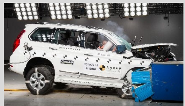
Frontal offset test at 64km/h
