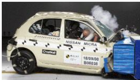
Offset crash test at 64km/hr
