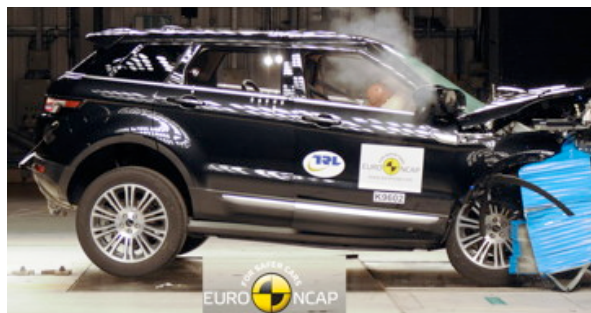
Offset crash test at 64km/h
