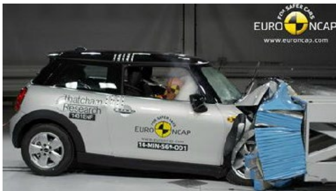
Frontal offset test at 64km/h
