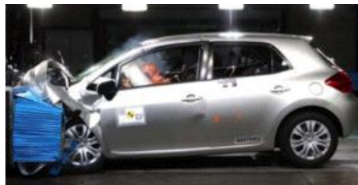
Offset crash test at 64km/hr
