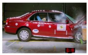
Offset crash test at 64km/h
