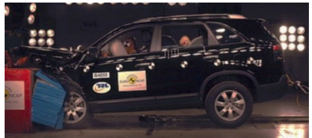
Offset crash test at 64km/h (Euro NCAP 2009)
