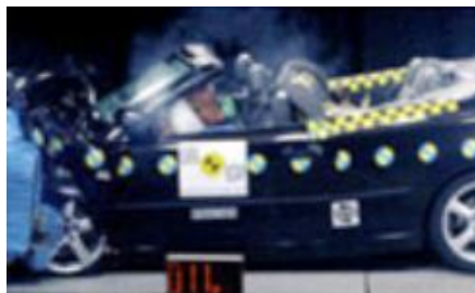
Offset crash test at 64km/hr
