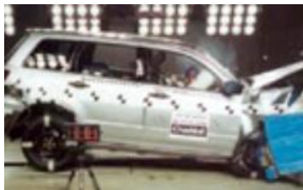
Offset crash test at 64km/hr
