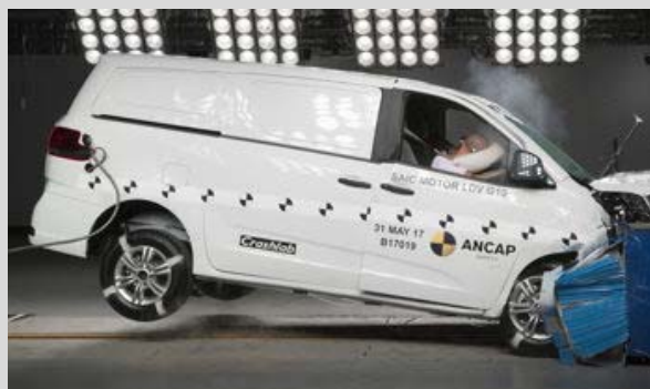
Frontal offset test at 64km/h
