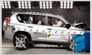
Frontal offset test at 64km/h
