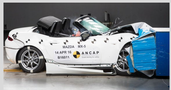
Frontal offset test at 64km/h
