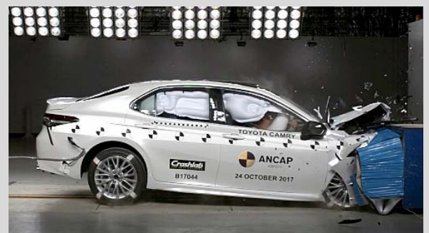
Frontal offset test at 64km/h
