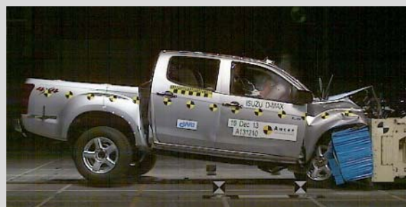
Frontal offset test at 64km/h
