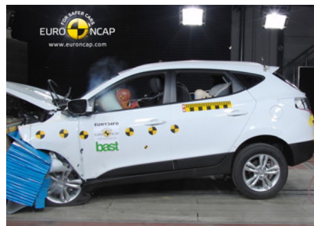
Offset crash test at 64km/h
