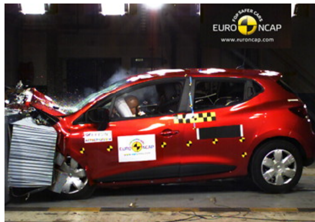
Frontal offset test at 64 km/h (Euro NCAP)
