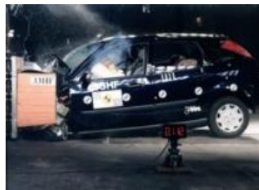
Offset crash test at 64km/hr
