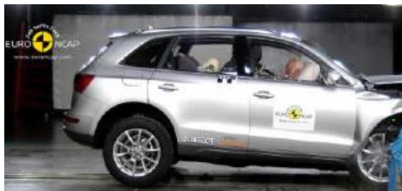
Offset crash test at 64km/hr
