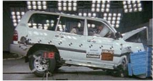
Offset crash test at 64km/hr
