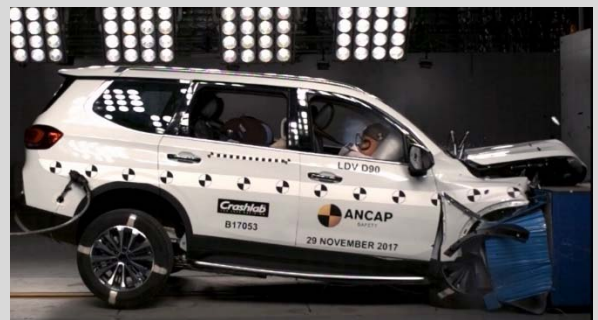
Frontal offset test at 64km/h
