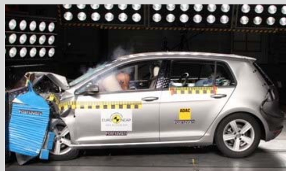
Frontal offset test at 64km/h
