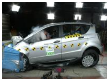
Offset crash test at 64km/hr
