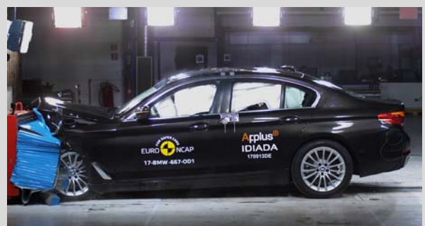
Frontal offset test at 64km/h
