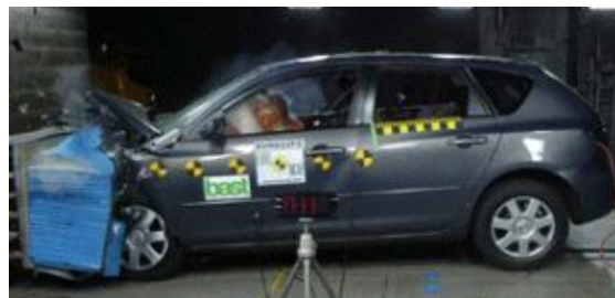
Offset crash test at 64km/hr
