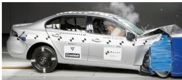
Offset crash test at 64km/h (2008)
