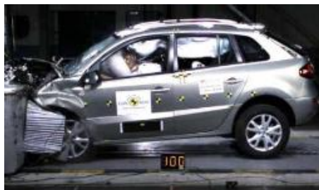
Offset crash test at 64km/hr
