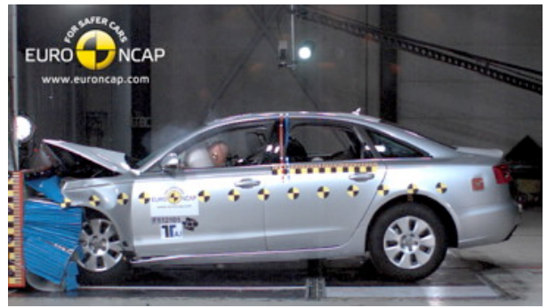
Offset crash test at 64km/h
