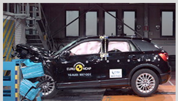
Frontal offset test at 64km/h
