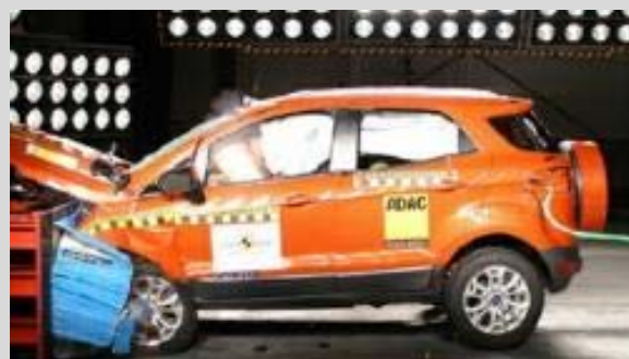
Frontal offset test at 64km/h
