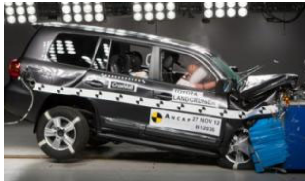
Frontal offset test at 64 km/h
