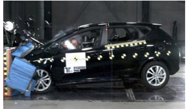
Frontal offset test at 64 km/h (5 door hatch - Euro NCAP)
