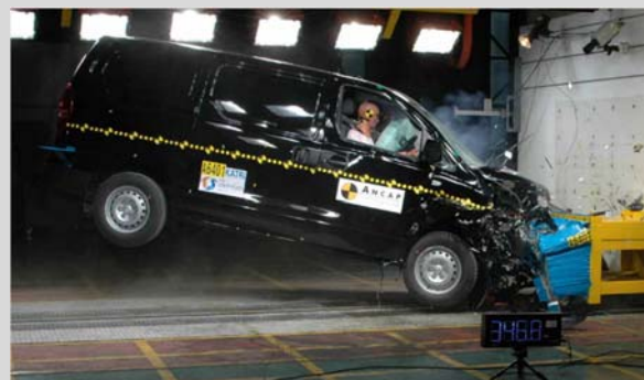
Frontal offset test at 64km/h
