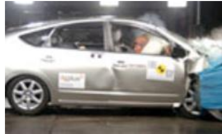
Offset crash test at 64km/hr
