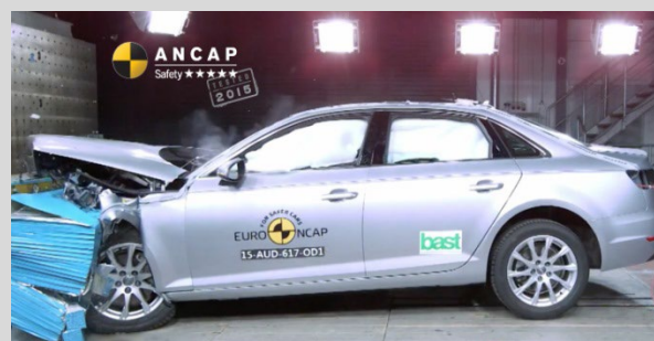
Frontal offset test at 64km/h (Audi A4 pictured)
