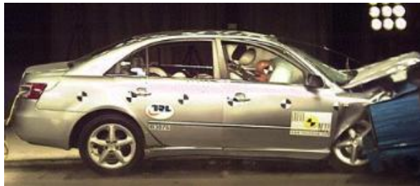
Offset crash test at 64km/hr
