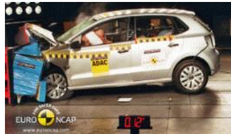
Offset crash test at 64km/hr
