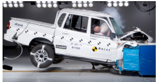
Offset crash test at 64km/h
