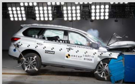
Frontal offset test at 64km/h
