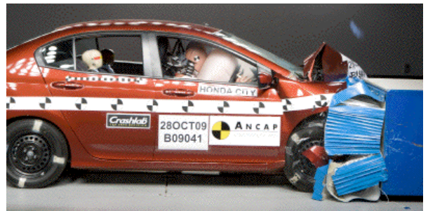
Offset crash test at 64km/h
